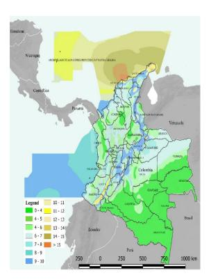
Figure 2. Wind speed map 2000 - 2010 Elaborated with IDEAM's data
