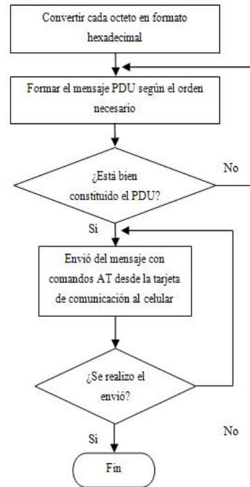
Figure 7. PDU Construction
