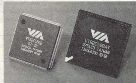
**Figura 1.** ChipSet VT82C598AT (North Bridge), VT82C586B (South Bridge)
