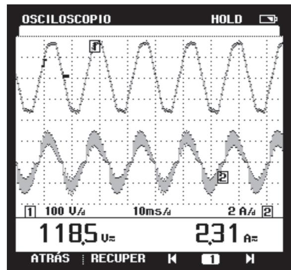
**Figure 6.** Input voltage and current in prototype with scheme of control in closed loop (THD = 18,32%).
