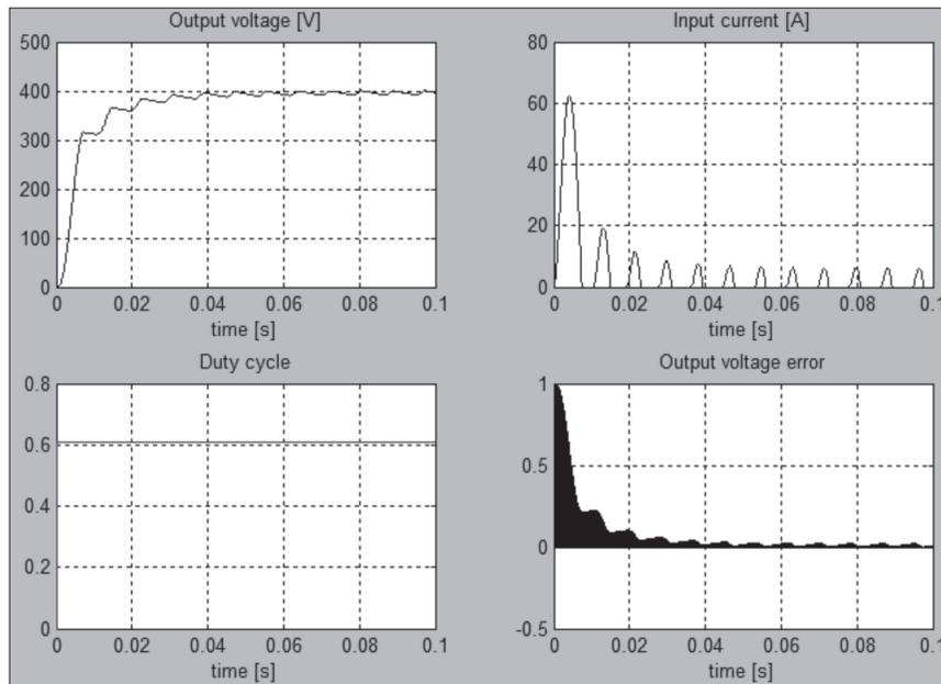
**Figure 2.** Step response of boost converter (simulation open loop). Starting current greater to 60 A.
