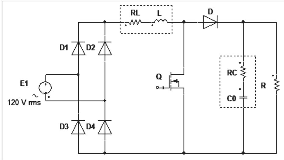
**Figure 1.** The DC/DC boost converter. This switching-mode converter contain two semiconductor switches (Q and D) and one energy storage element (L). The output capacitor (Co) works as filter.
