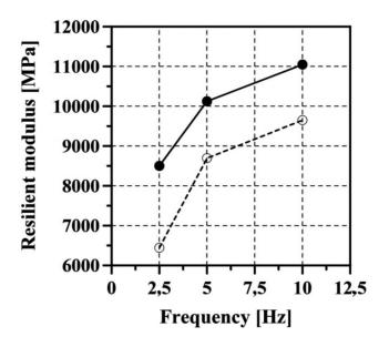
**Figure 5.** Evolution of the Resilient Modulus at 5°C (HMA-25 and WMA-25)
