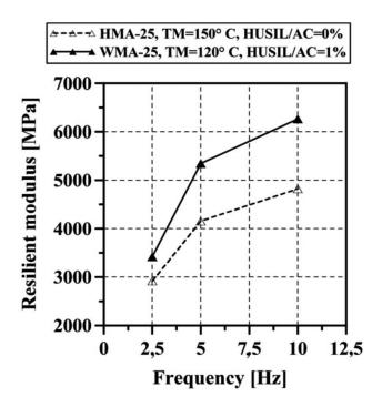
**Figure 6.** Evolution of the Resilient Modulus at 15°C (HMA-25 and WMA-25)
