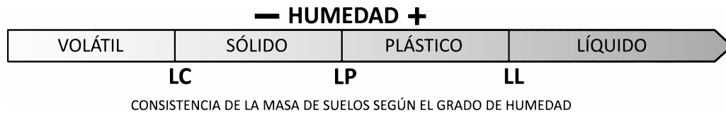
Figure 2. Theoretical consistency of the soil mass according to the moisture content
