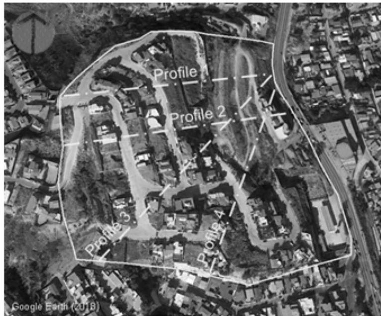
Figure 6. Profiles used for slope stability analysis.
