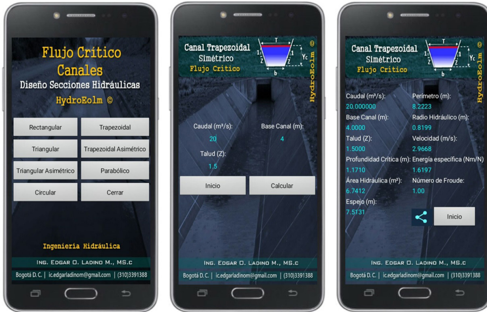
Figure 15. Exercise 3.5, Hydraulics of channels, Gilberto Sotelo (Application Critical depth calculation) Source: Authors.
