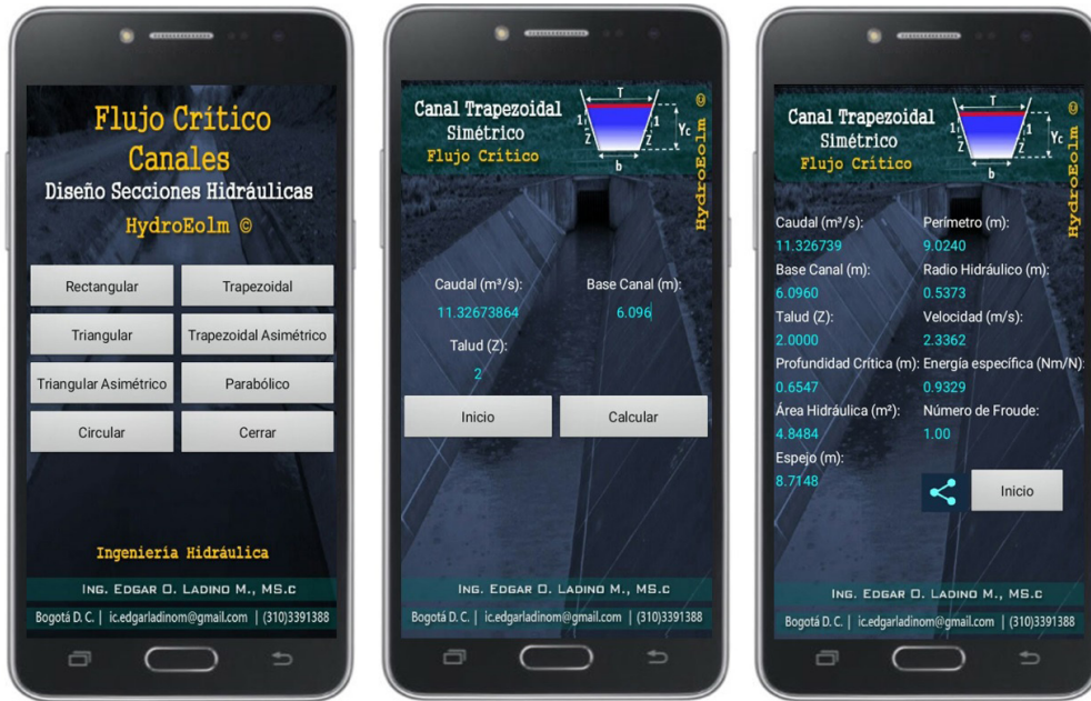
Figure 16. Exercise 4.2, Hydraulics of open channels, Ven Te Chow (Application Critical depth calculation) Source: Authors.
