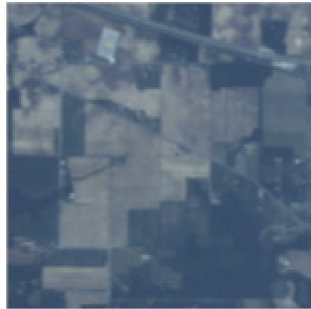
Figura 3. Composition RGB for Indian Pines. Red plane: band 30 (654.5 nm), Green plane: band 20 (557.7 nm) and Blue plane: band 9 (451.3 nm).
