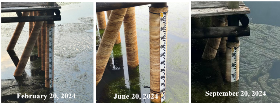
Figure 2. Limnimeter installed in the EEFL
