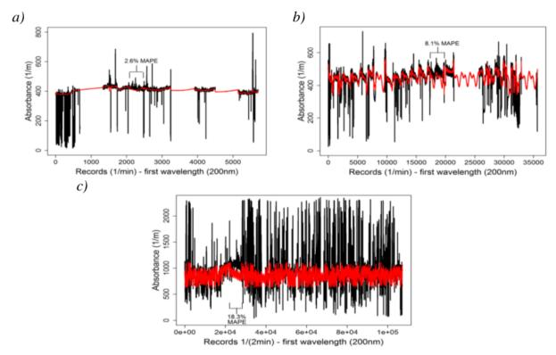
**Figure 5.** Resulting time series and MAPE values for all three study sites after removal a selecting range values and applying the proposed procedure to Salitre-WWTP (a), GPS (b) and San Fernando-WWTP (c) (self-authorship)
