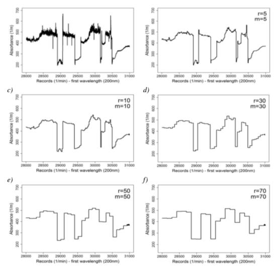
**Figure 3.** Comparison of different r and m Winsorising parameter values for the GPS Absorbance time series (section spanning values 28000 to 31000) with original (a), r = m = 5 selected value (b), r = m = 10 selected value (c), r = m = 30 selected value (d) and r = m = 50 selected value (e), r = m = 70 selected value (f) (self-authorship)
