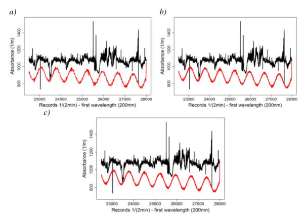
**Figure 6.** Resulting time series and MAPE values for San Fernando WWTP study site after removal a selecting range values and applying the proposed procedure for 5% (a), 10% (b) and 20% (c) of most relevant harmonics respectively (self-authorship)
