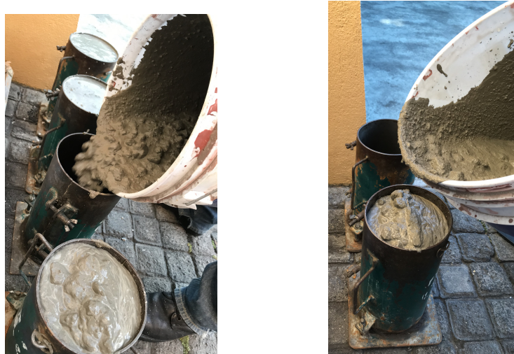
Figure 4. Pouring the concrete mixture into the molds
