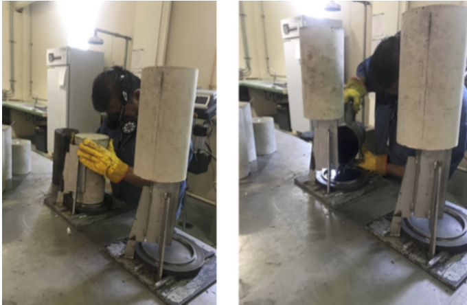
Figure 8. Placement of sulfur
