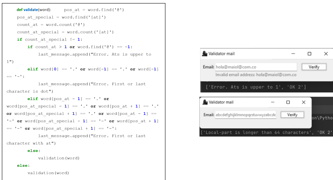
Figure 4. Validation of the number of @ and of characters (a) with their corresponding results for each case (b)
