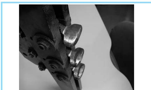
Figure 11 Worn fixed contacts selector switch
