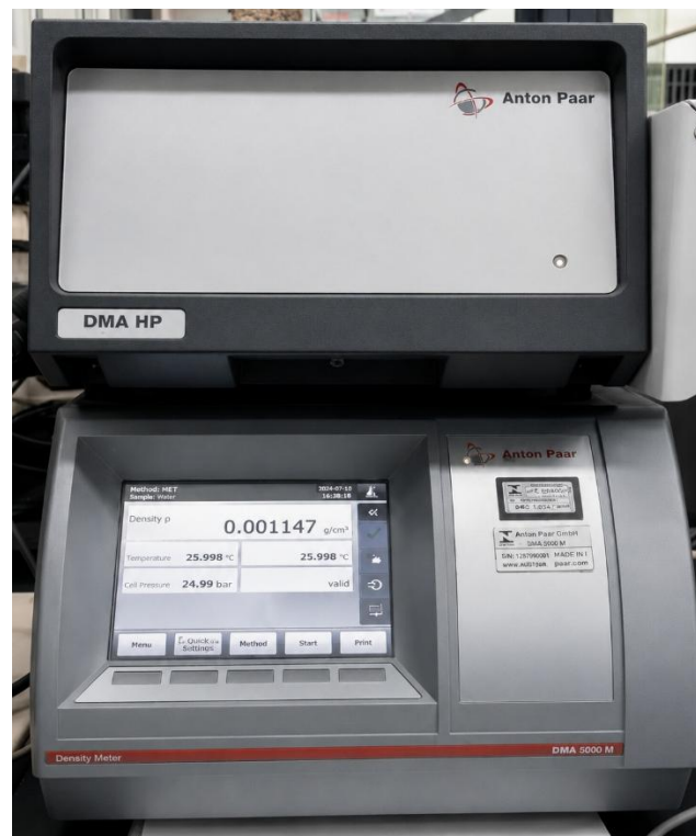
Figure 2. Pressure cell (DMA HP) and digital densimeter (DMA 5000M) (Source: Inmetro/Laflu)
