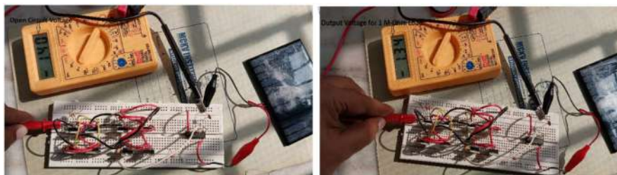
Figure 7. Voltages obtained for a 1 M \Omega load resistance
