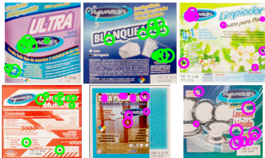
Figure 7. Interest points selected by the SURF algorithm on the labels of the six selected products.
