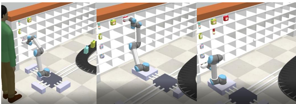
Figure 10. Execution of the process of classification and arrangement of products on the shelf.
