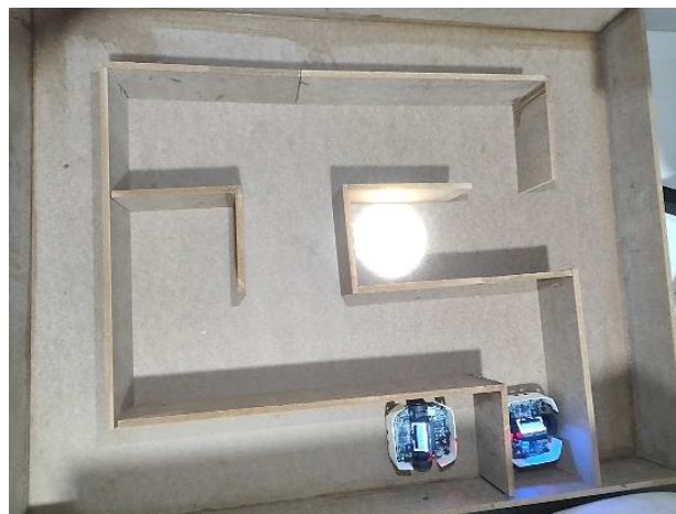
Fig. 1. Experimental maze used for swarm robot navigation and clustering tests.
