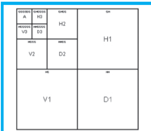
Figure 5. Wavelet decomposition. A indicates approximation, H horizontal, V Vertical and D Diagonal. The top sequences on each subband means a series of convolutions with the H (high pass filter) and G (low pass filter).
