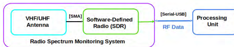
Figure 15. Fundamental constituent components of the SIGINT module, such as the VHF/UHF antenna, SDR (26), and the process unit.
