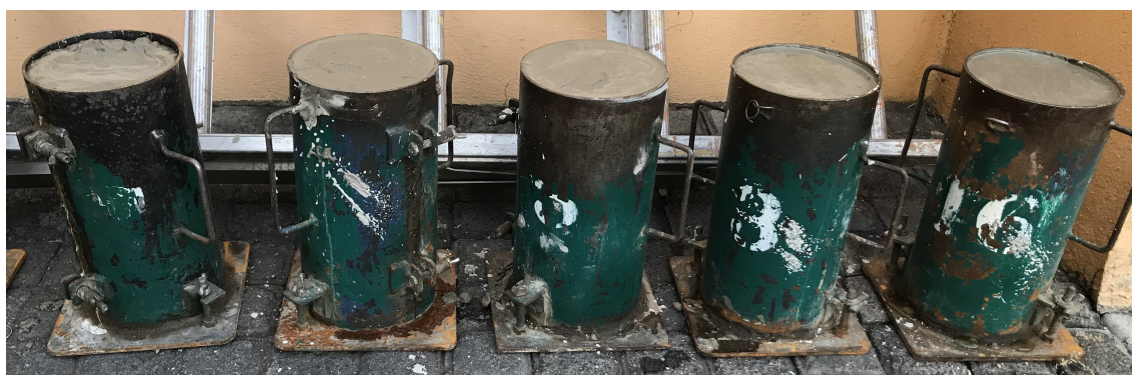
Figure 5. Molds in the drying process
