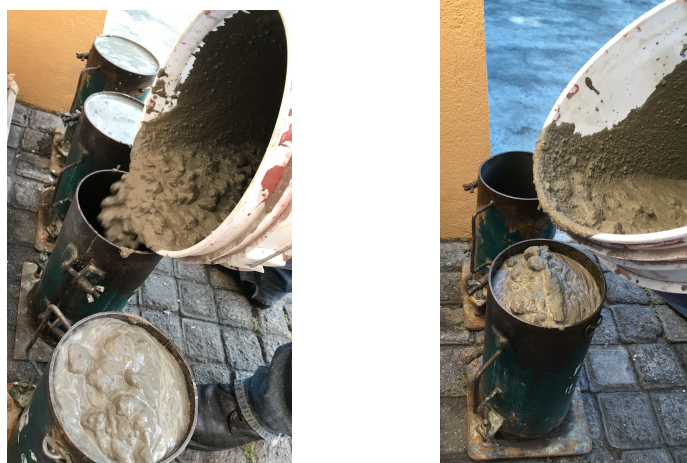
Figure 4. Pouring the concrete mixture into the molds
