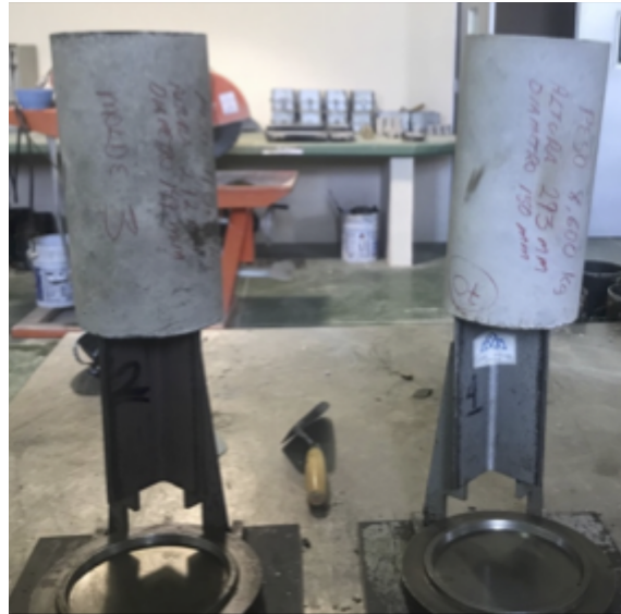
Figure 7. Arrangement of specimens prior to placement of sulfur
