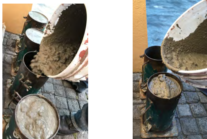
Figure 4. Pouring the concrete mixture into the molds
