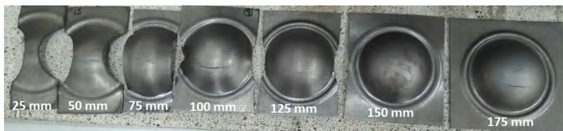
Figure 6. The seven SG325 steel specimens deformed to failure
