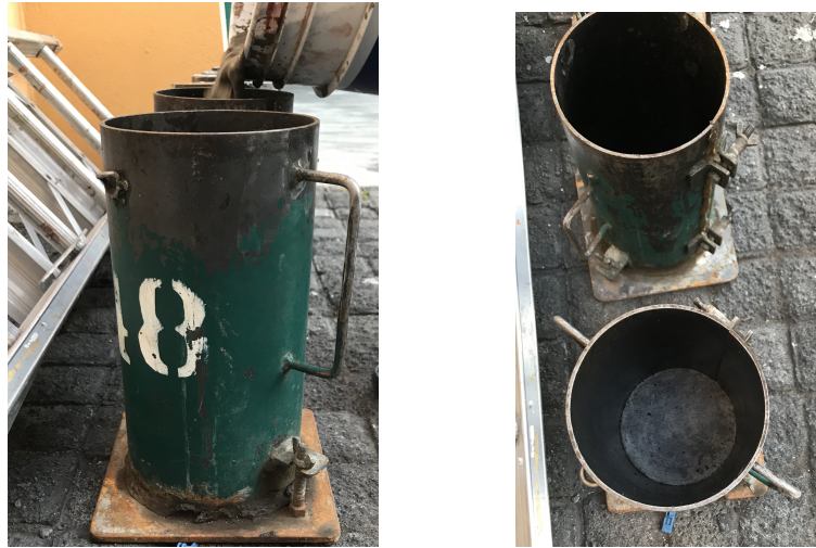
Figure 2. Molds used to make the specimens
