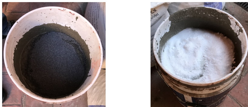
Figure 3. Concrete with fly ash (left) and nanosilica in concrete (right)
