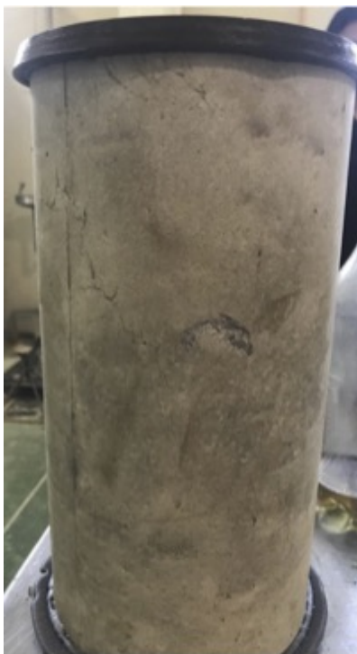
Figure 12. Fractured specimen after being subjected to the strength test
