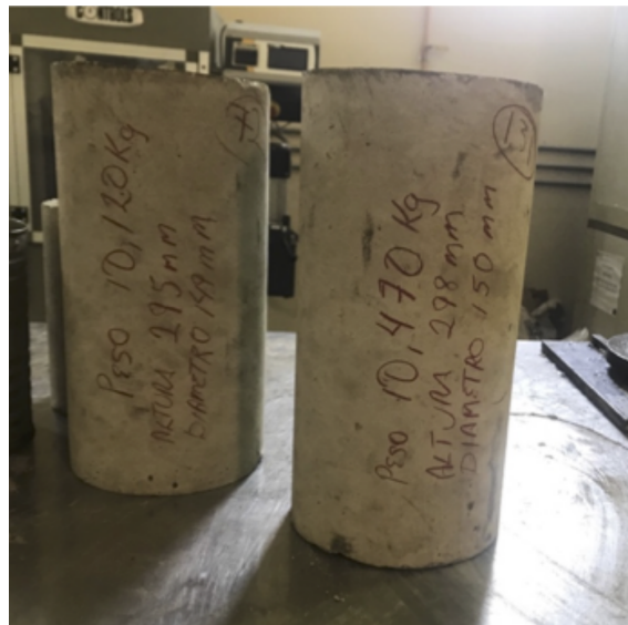
Figure 6. Demolded and labeled specimens
