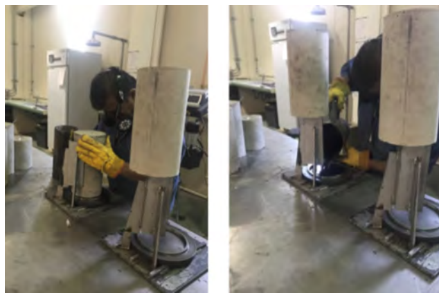
Figure 8. Placement of sulfur
