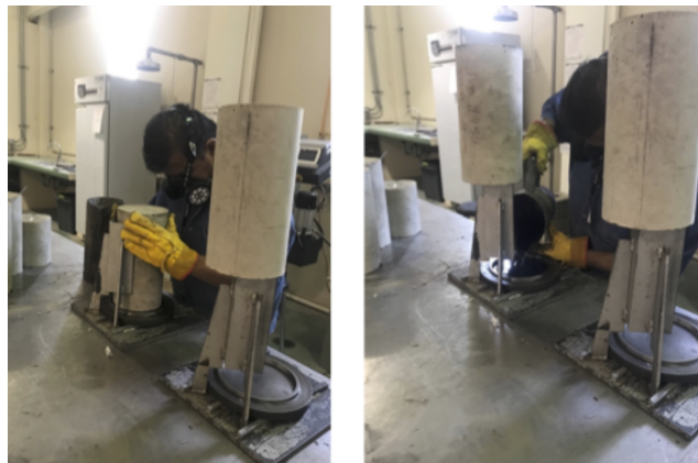
Figure 8. Placement of sulfur
