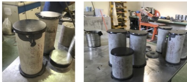
Figure 9. Specimen ready for resistance tests
