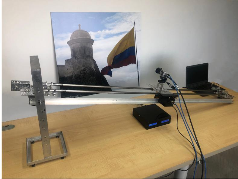
**Figure 6.** Rig setup to generate uniformly accelerated motion-blurred images
