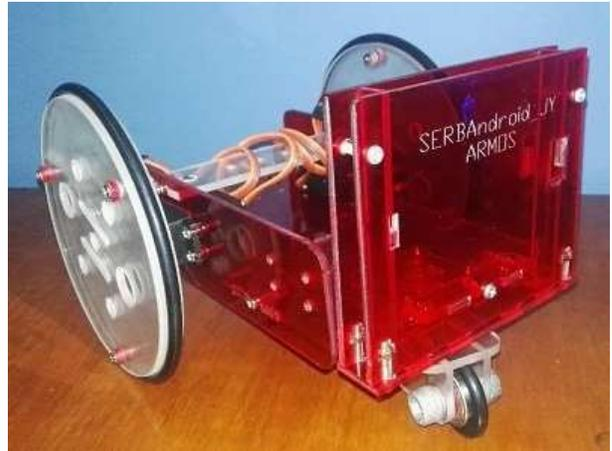
Figure 30. SERB robot fully assembled with smartphone holder.
