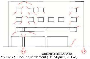
The damage caused by the settlements are the cracks, usually these cracks are inclined and directed to the point where is the settlement, have an arc shape and appear at all levels of the construction.
