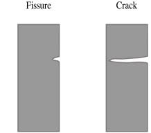
Figure 5. Fissure and crack comparison.
