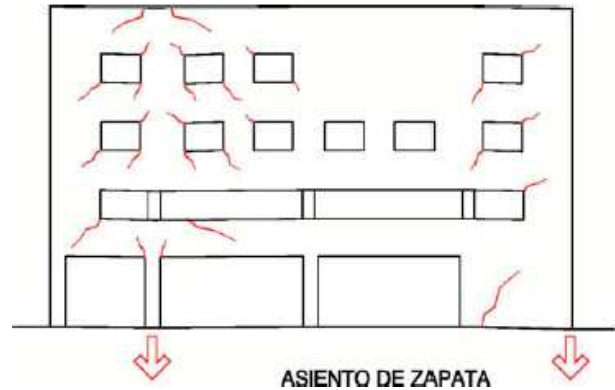
Figure 15. Footing settlement (De Miguel, 2017d).
