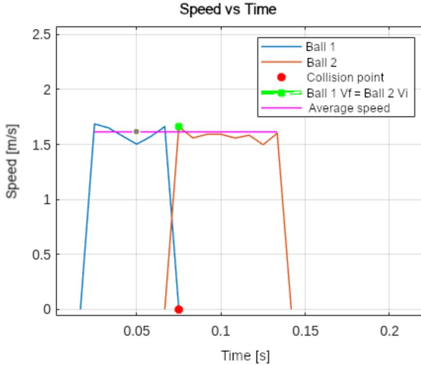
enough to affect the nature of the collision. On average the velocity is  $v = 1.6149$  m/s (Fig. 9).
