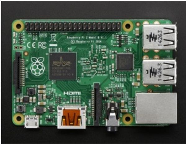
Figura 6. Raspberry Pi 2 Modelo B (Adafruit, 2015).
