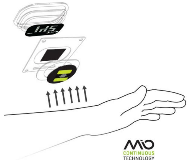
Figura 3. Sistema sensado Mio Continuous Technology (MIO, 2015).
