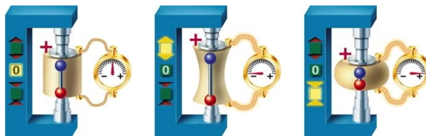
Figure 1. Piezoelectric effect schematically.
