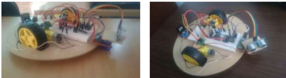
Figure 3: Prototype of differential mobile robot developed.
