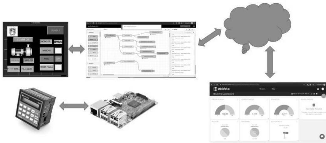
**Figure 7.** Information flow from PLC to dashboard. Source: own.
