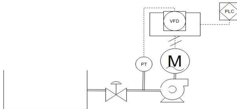
**Figure 3.** P&ID layout of system instruments. Source: own.
