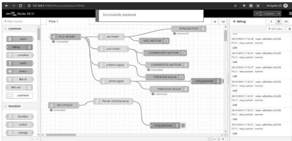
**Figure 8.** Node-RED flows system for TCP protocol. Source: own.
