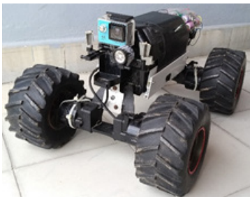
Figure 1. Teleoperated vehicle based on Arduino
