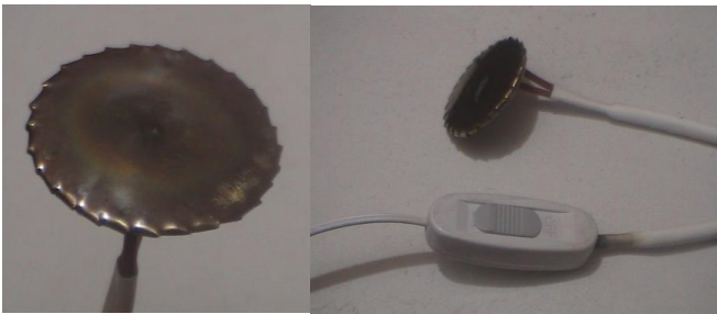
Figure 4. Electrical resistance of the heating system.
