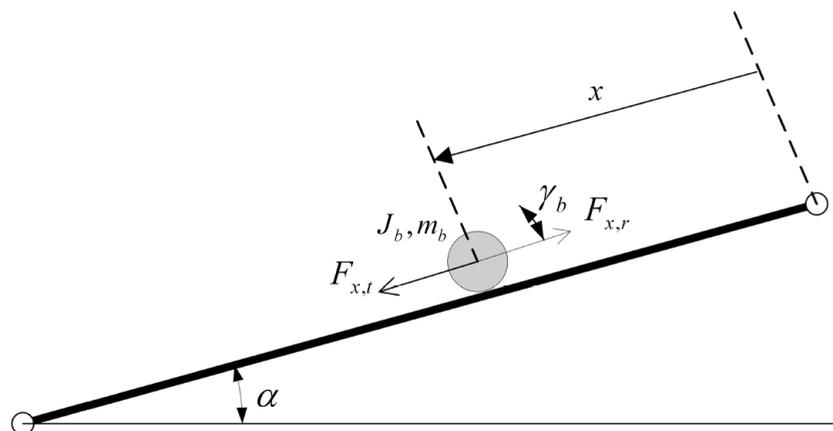
Starting from equation (1) given by Newton’s second law, equation (2) related to the nonlinear dynamic model, which describes the motion of the ball along the beam, is derived; the parameters used for the modeling of the system are shown in Table 1.
