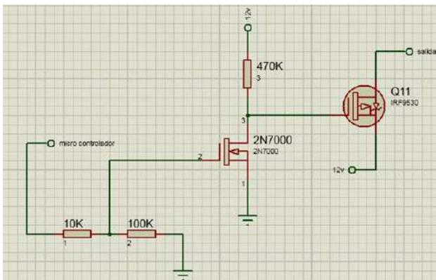
**Figure 10.** Circuit schematic, managed with power MOSFET for the injectors control. Source: own.
