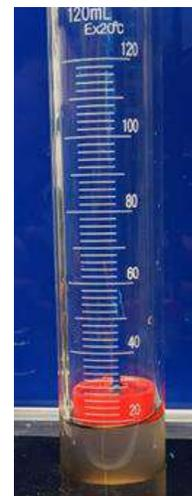
**Figure 22.** Liquid quantity deposited by an injector in good condition. Source: own.
