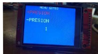
**Figure 17.** Leak menu in manual control. Source own.
