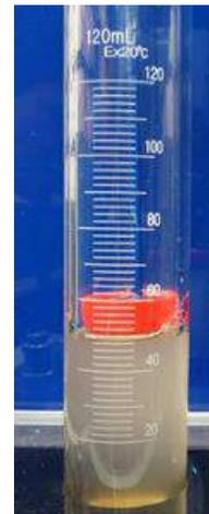
**Figure 21.** Liquid quantity deposited by an overconsuming injector Source: own.
