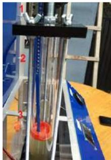
**Figure 15.** Float type level sensor: 1-Encoder, 2-segmented bar, 3- float. Source: own.
