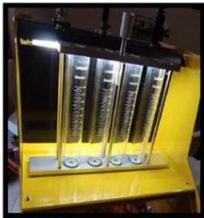
**Figure 3.** Gasoline injectors tester activated and controlled via Wi-Fi. [10].
