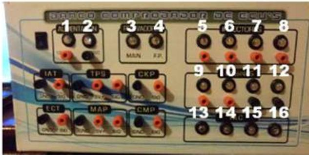
**Figure 2.** Test stand for electronic vehicle control unit with electronic injection systems. [9].
