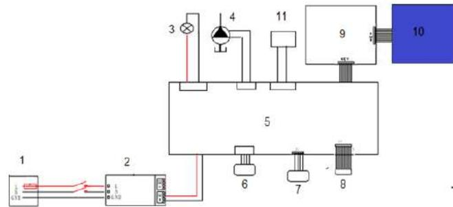
Figure 8. Electrical system: 1) AC power, 2) DC power supply, 3) backlighting, 4) pump, 5) psoc micro controlled system, 6) sensors, 7) solenoid valves, 8) injectors, 9) micro controlled system 2, 10) control panel, 11) wireless communication. Source: own.
