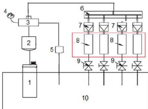
Figure 7. Hydraulic system: 1) gasoline pump, 2) filter, 3) tee, 4) manometer 5) return, 6) rail, 7) injectors, 8) measuring pipes, 9) solenoid valves, 10) tank. Source: own.
