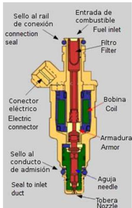
**Figure 1.** Parts and internal injector scheme. [7]
