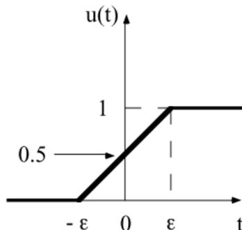
In the unitary step derivative, in the generalized distributional sense, the length tends to 0 and the amplitude tends to  $\infty$ . In addition, the area between the signal and the abscissa axis remains constant when  $\varepsilon$  tends to 0, figure 3.
