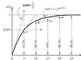
As it can be seen, the response is a growing exponential signal that originates in 0 and stabilizes in 1. Based on this behavior, characteristics such as the time constant, the signal  $c(t)$  that describes the response, the amplitude in which the system stabilizes and the stabilization time can be calculated depending on the criterion taken, which can be between  $3T$  and  $5T$ .
