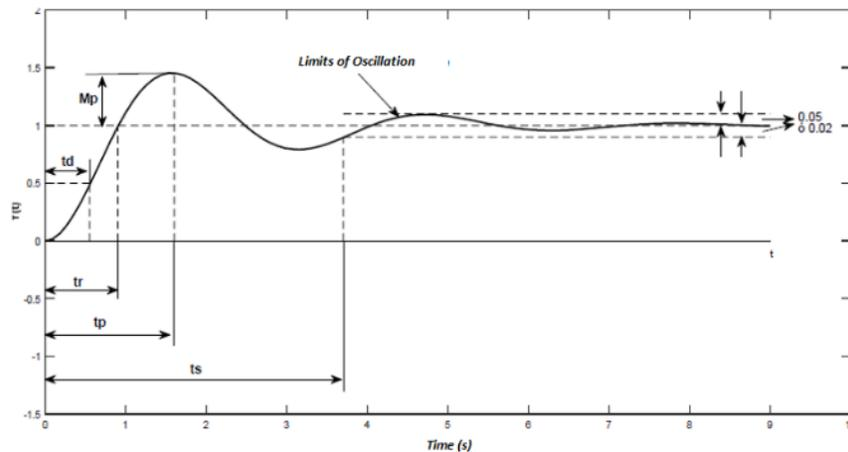
It can be seen that the signal response is a signal used to calculate important characteristic values in second order systems as maximum on impulse ( $M_P$ ), stabilization time ( $t_S$ ), peak time ( $t_P$ ), delay time ( $t_d$ ) and rise time ( $t_r$ ).
