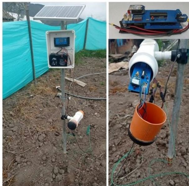
Figure 2. Assembly of the intelligent irrigation system prototype in the field.
