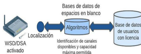
Figure 1: TVWS database access method. [16].
