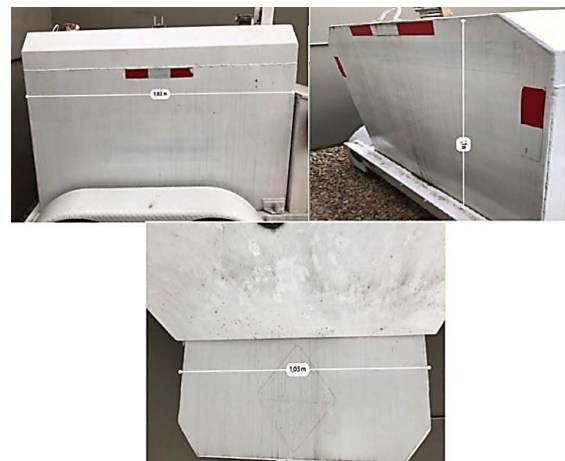
Figure 9. ACPM storage tank measurements. [16]
