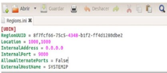
Figure 3. Regions view with location, internal address, port and the name of the UDIN server, the Regions ID is composed by a hexadecimal number unique in the world.
