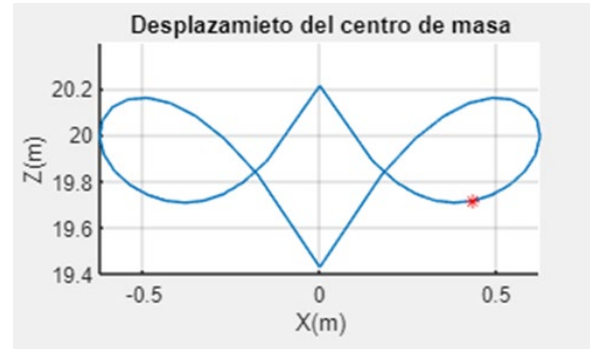
Figure 15. Behavior of the center of mass in walking locomotion.
