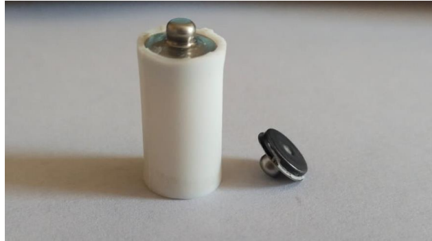
Figure 1. Dials used for EIS measurement in cocoa oil samples.
