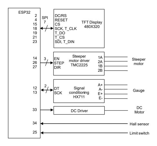
Figure 1 shows the connection of an ESP32 microcontroller to the selected electronic devices to measure viscosity according to the concentric cylinder principle [2]. Describing each of the functional blocks in Figure 1:
