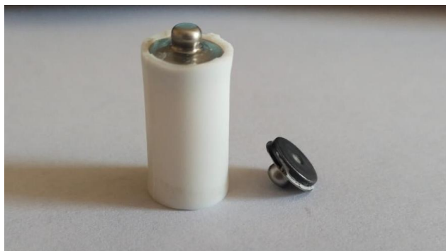
Figure 1. Electrodes used for EIS measurements in cocoa butter samples.
