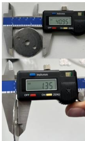
Figure 1. Measurements of the stainless-steel washers.
