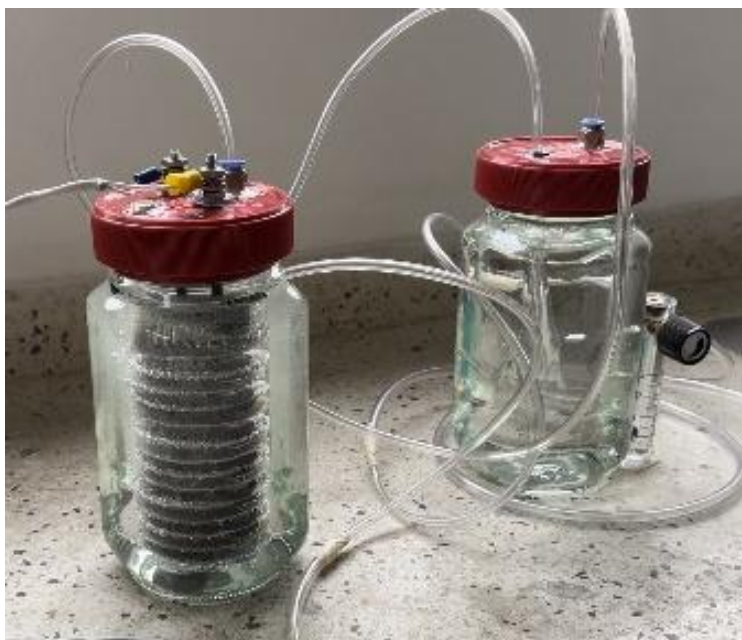
Figure 4 First prototype Hydrogen Generator.
