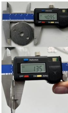
Figure 1. Measurements of the stainless-steel washers.
