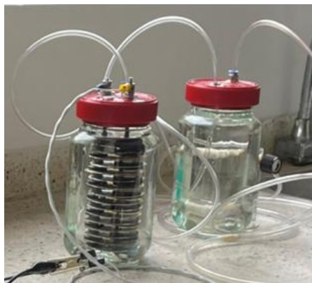
Figure 2 Hydrogen Generator and Bubbler
