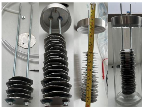
Figure 6 Assembly of the second electrode.
